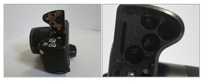
• Open the battery cover and remove the AA batteries from the camera if any are inserted.
