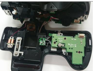
Use a Plastic Opening Tool to carefully remove the top of the camera.
