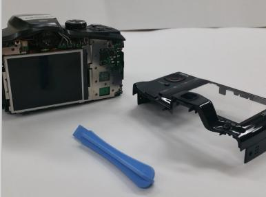
Use a Plastic Opening Tool to remove the back of the camera
