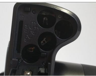
Open the battery cover and remove the AA batteries from the camera if any are inserted.
