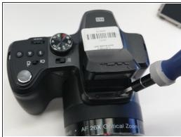
• Open the flash compartment and remove two (2) **3mm** screws.
