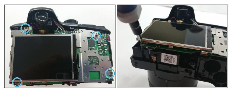
Once the back cover is removed locate the four 3mm screws holding the screen and the metal brace to the circuit board
