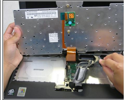
**⚠ Be careful not to pull out the keyboard carelessly; there is a connector underneath it!**
