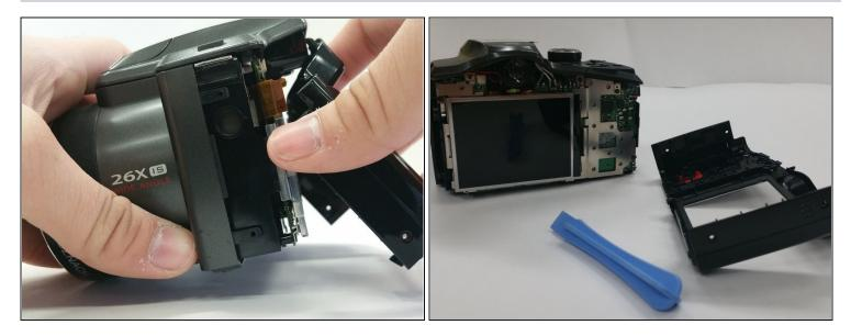
• Use a Plastic Opening Tool to remove the back of the camera and pull gently on the cover to remove the cover
