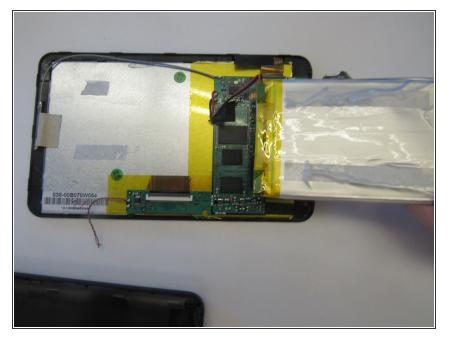
Replace the damaged or malfunctioning battery with the new battery and wires. The new battery must be stuck back into its original place using thermal tape.
