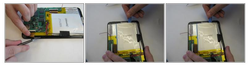
• Remove the battery pack by carefully prying the battery back from the front cover. Then, remove the wires connecting the battery to the motherboard at the motherboard using the tweezers.
