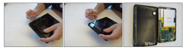
• Remove the back cover with a plastic opening tool, exposing the battery and motherboard.
