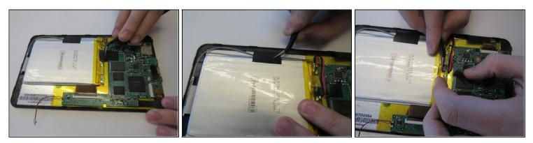
• Remove the two black tape strips from the battery pack.
