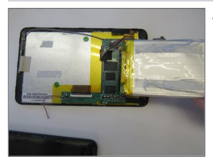
Replace the damaged or malfunctioning battery with the new battery and wires. The new battery must be stuck back into its original place using thermal tape.
