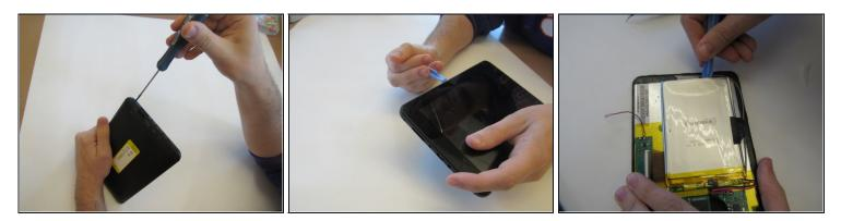
• Remove the two 2.4 mm x 4 mm Phillips #00 screws from the bottom of the tablet.
