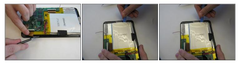
• Remove the battery pack by carefully prying the battery back from the front cover. Then, remove the wires connecting the battery to the motherboard at the motherboard using the <u>tweezers</u>.
