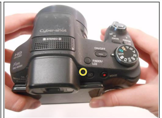
**i** Use the Phillips screwdriver size #00 to remove the 1.59mm #00 screws.
