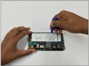
• Using the plastic opening tool, apply an upward force to detach the battery and the tab attached to it.
