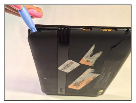
1. Using the plastic opening tool, carefully insert the opening tool on all four corners of the Kindle Fire and lift up until you hear a slight popping noise.
