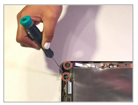
• Using the Phillips #00 screwdriver, unscrew the two 3mm screws.
