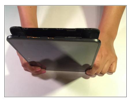
Using the plastic opening tool, start from one corner and go around the Kindle Fire using the tool in a down
