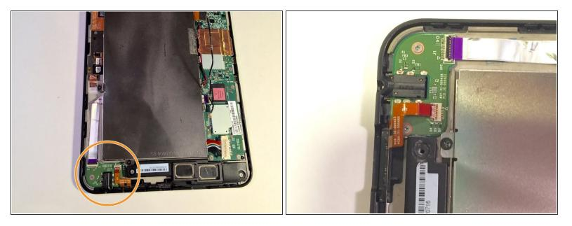
• Locate the headphone jack, which is by the volume buttons on the vertical edge of the Kindle.
