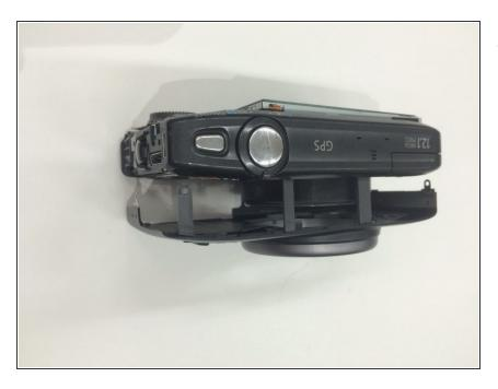
After removing exterior screws, gently lift off the front face plate.
