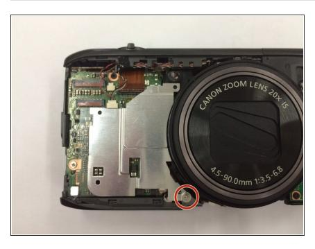
Remove 1 (6 mm) Screw from the bottom of the silver metal plate. The screw is also silver
