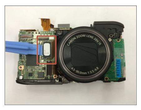
Use the blue spludger tool to gently unplug the last ribbon cable that is attached to the motherboard.
