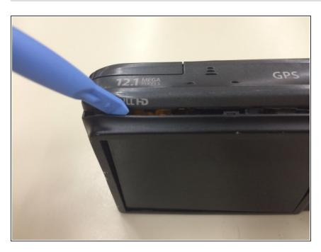
Use spludger tool or small flathead screw driver to gently lift and remove back face plate.
