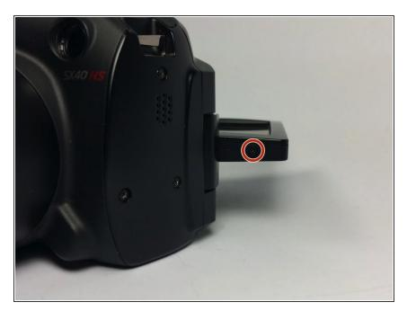
Partially close the screen and rotate it 90 degrees until the screen is facing upwards (photo view from the left front of the camera). Remove the 4mm black screw, indicated in the picture, with a Phillips #00 screwdriver.
