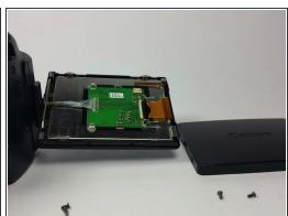
This is what you should see after removing the LCD screen cover. Replace the LCD screen cover if damaged.
