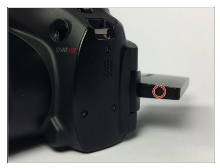
Rotate the screen 180 degrees until the monitor is facing downwards.
