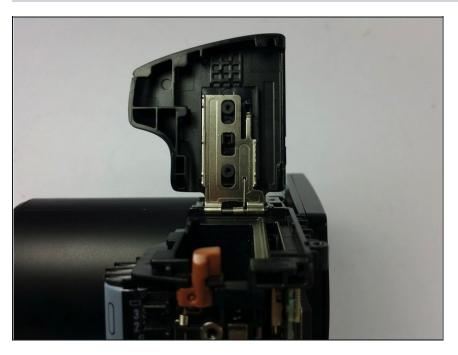
Remove the battery compartment cover from the metal bracket.
