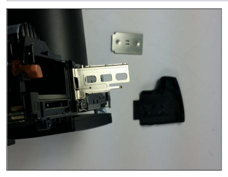
Replace either the internal metal battery contact or external battery compartment cover.
