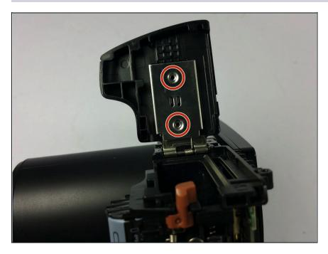
Remove the two circled 2mm screws with a Phillips #00 screwdriver.
