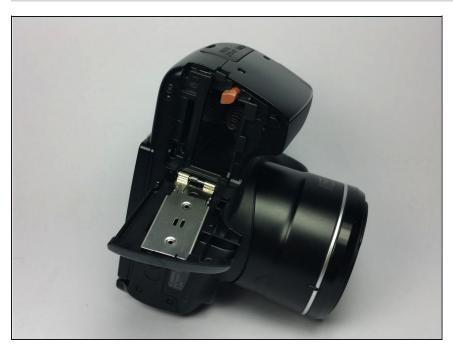
Slide the metal battery contact away from the battery compartment cover.
