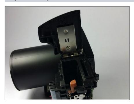
Orient the camera so that the bottom of the camera is facing up and open the battery compartment.
