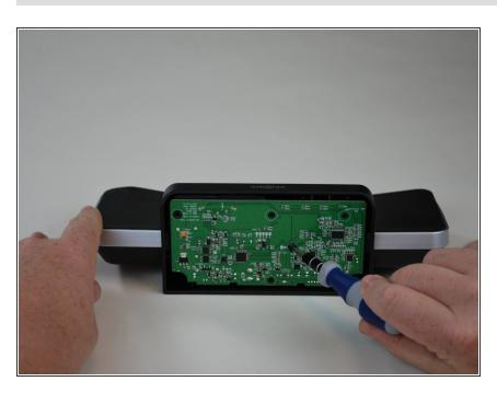
Unscrew the 9.5mm screw located near the center of the motherboard with a Phillips head screw driver.
