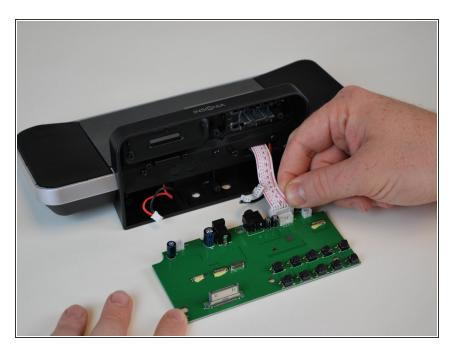
Remove the LCD screen plug last.
