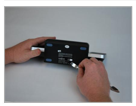
Peel back the adhesive sticker using a metal spudger and remove the 11mm screw beneath the sticker with a Phillips head screw driver.
