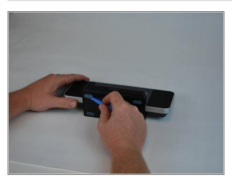
Using a plastic spudger, peel off the adhesive gel stoppers.
