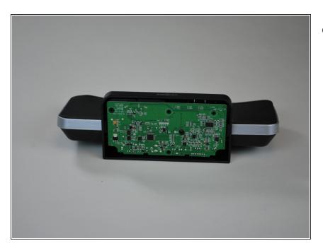
Remove the bottom of the device to reveal the motherboard.
