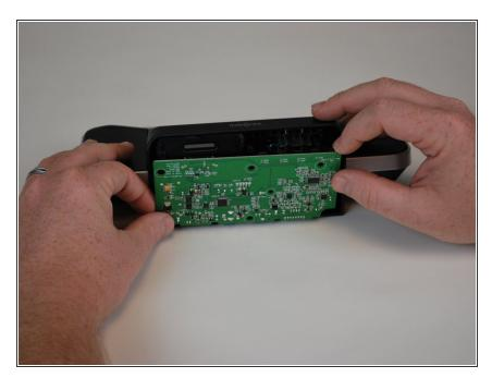
Lift the motherboard from the device and lie it face down. Beware of the cables plugged in on the back side
