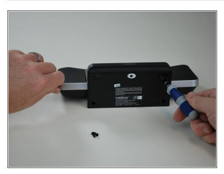
Unscrew the six 11mm screws with a Phillips head screw driver.
