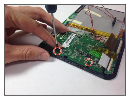
Remove the 2 Phillips #00 4.5 mm screws from the motherboard.
