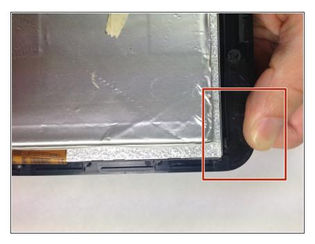
Gently pull the front case clips down and off of the back of the screen for all of the remaining clips
