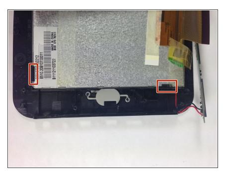
Gently pull the front case clips down and off of the back of the screen
