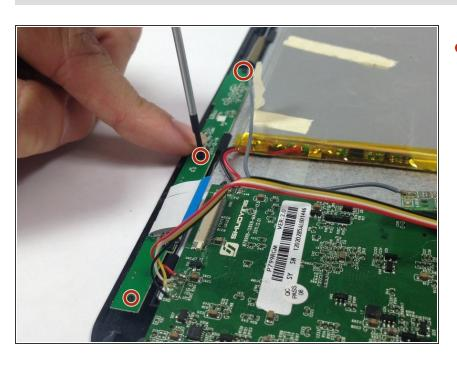
Remove the 3 Phillips #00 4.5 mm screws from the side button array.
