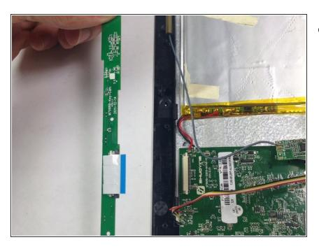
Remove the side button array from the device.
