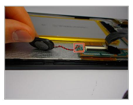
Gently peel back the black electrical tape covering the contact points between the speaker wires and the
