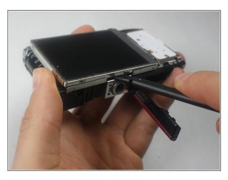
Raise the screen by wedging the spudger between the bottom of the screen and the mount hole.
