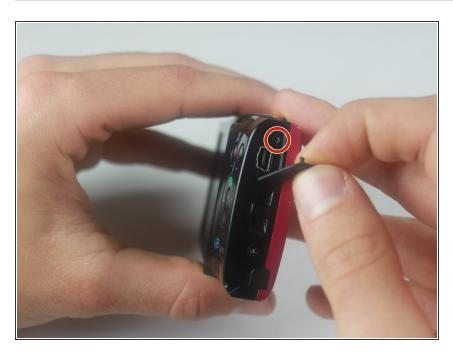
Open the A/V Out Digital port cover on the function button side to reveal a screw.
