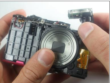
Remove the flash by gently rotating slightly back and forth and pulling up.
