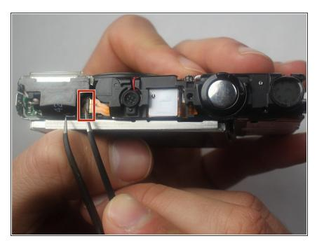
Use one side of the tweezers to raise the orange retaining flap on the zero insertion force (ZIF) connector to a vertical position.
