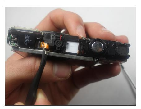
Gently pull the orange ribbon cable out of the ZIF connector using the tweezers.
