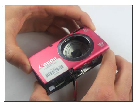
Pull the top of the front cover away from the camera by gripping the top of the front cover by the corners where the cover is still attached to the body.
