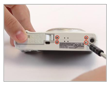
Remove the four 4mm screws from the bottom of the camera with a Phillips PH000 screwdriver.
