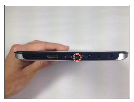
Remove the 4.6mm Phillips #00 screw at the base of the device.
