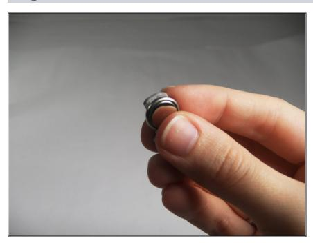
• Replace the internal battery.
