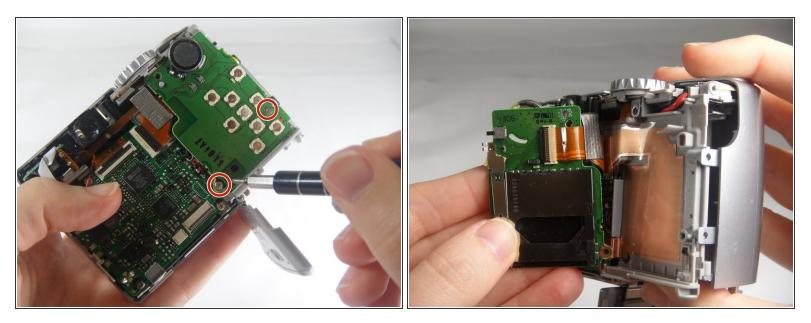
• Remove the two (2) 3.0 mm screws with the Phillips head #000 screwdriver.
