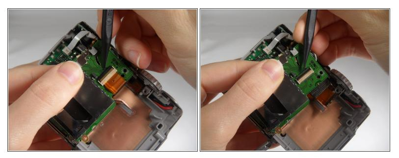
• Remove the orange ribbon from the clamp by using a Spudger to push the bar up.
