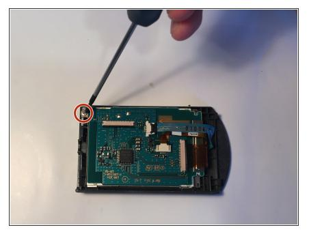
• Unscrew the 2mm Phillips #00 screw from the screen chip.
