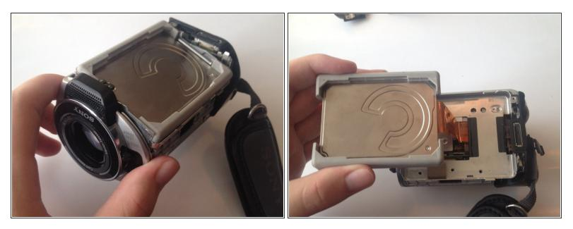
Lift the hard drive out of the camera by grasping the grey rubber mounting brackets and pulling them upwards.
