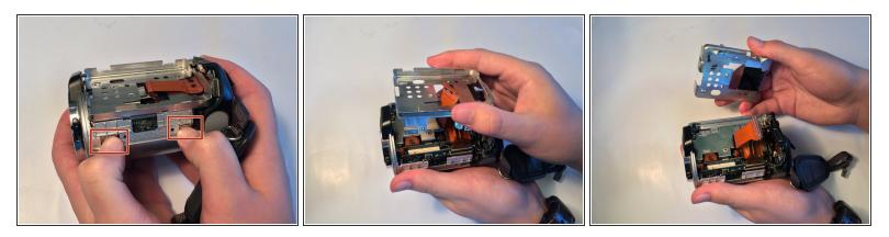
• Press in on the two tabs as shown and lift the metal plate up and off the camera.
