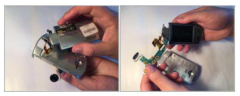
• Remove the screen from the plastic case by pulling the flex cable and sound chip through the hole in the case.
