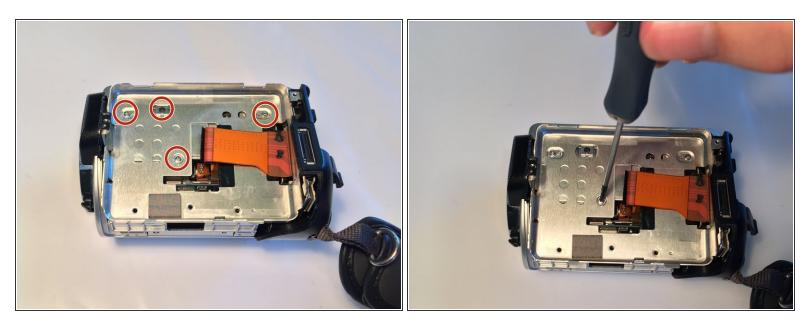
• Remove the four 3mm Phillips #00 screws from under the hard drive.
