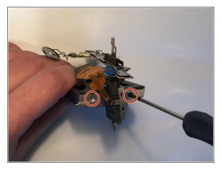
Turn the hinge sideways and remove the two 4mm Phillips #00 screws from the side of the screen.
