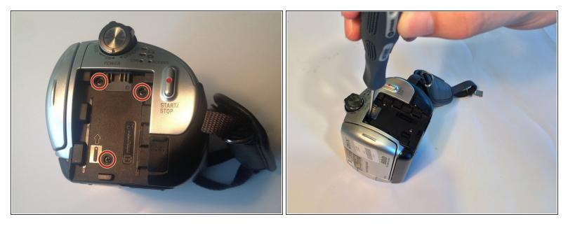
Remove the battery, and use the Phillips #00 precision screwdriver to then remove the three 3mm Phillips #00 screws under the battery.
