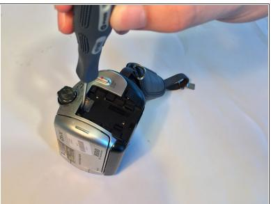
Remove the battery, and use the Phillips #00 precision screwdriver to then remove the three 3mm
