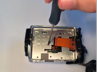
Remove the four 3mm Phillips #00 screws from under the hard drive.
