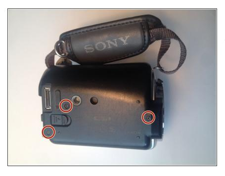
Remove the three 3mm #00 Phillips screws on the bottom of the camera.
