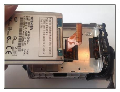
Carefully unplug the flex cable from the hard drive.
