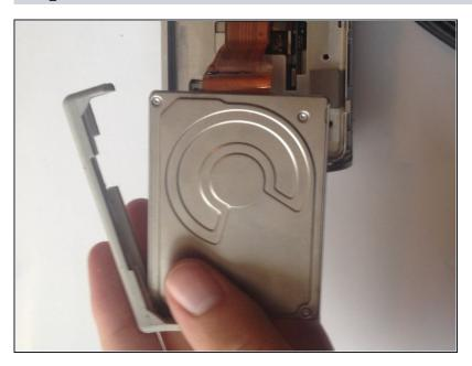
Remove the rubber mounting brackets by pulling them off the hard drive.
