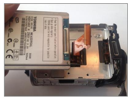
• Carefully unplug the flex cable from the hard drive.
