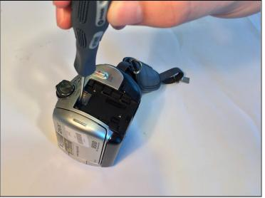
Remove the battery, and use the Phillips #00 precision screwdriver to then remove the three 3mm Phillips #00 screws under the battery.
