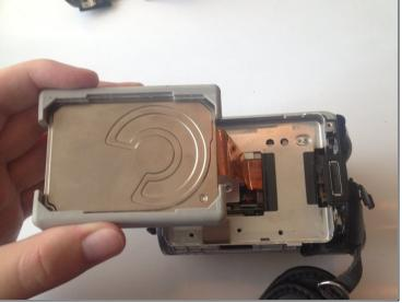
• Lift the hard drive out of the camera by grasping the grey rubber mounting brackets and pulling them upwards.
