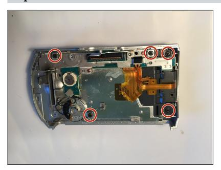
Remove the 5 3mm Phillips #00 Screws from the screen assembly.
