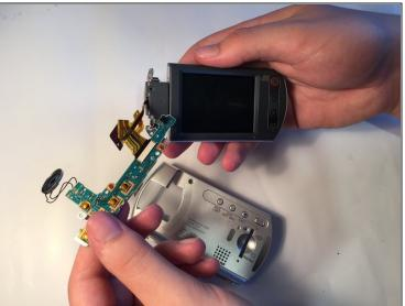
• Remove the screen from the plastic case by pulling the flex cable and sound chip through the hole in the case.
