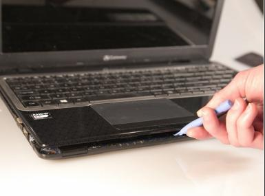
Separate the bottom panel from the touchpad assembly by inserting a plastic opening tool between them on all four sides.
