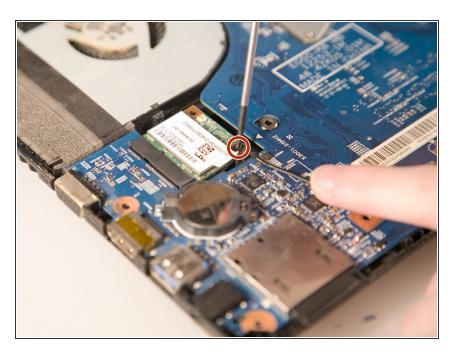
Remove the one 2.9 mm Phillips #00 screw holding down the wireless card in place.
