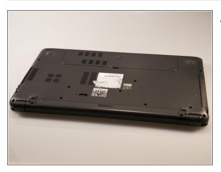
Flip the device over onto its backside in order to access the battery.
