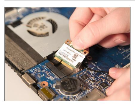
After the screw is removed, the card will spring upwards slightly. Pull out the old wireless card from its port.
