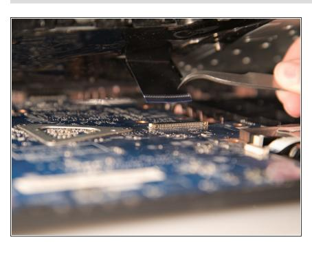
Pull black ribbon wire from port using tweezers in order to completely separate touchpad assembly from bottom assembly.
