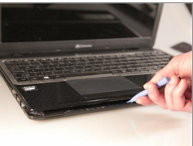
Separate the bottom panel from the touchpad assembly by inserting a plastic opening tool between them on all four sides.
