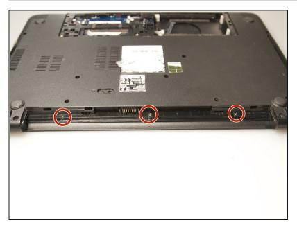
Remove three 2.9 mm Phillips #00 screws from the battery compartment.
