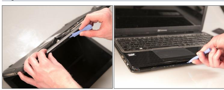
• Separate the bottom panel from the touchpad assembly by inserting a plastic opening tool between them on all four sides.
