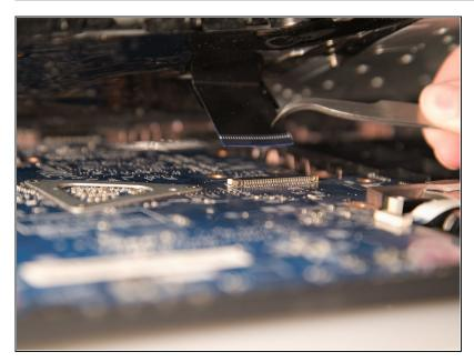
Pull black ribbon wire from port using tweezers in order to completely separate touchpad assembly from bottom assembly.
