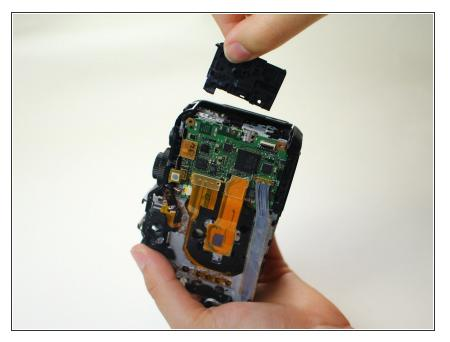
Insert the new HDMI port until you hear a click on both sides, ensuring the holes match up with the ports on the camera.
