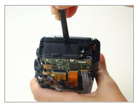
On the right side of the camera looking from the back, locate the HDMI port and use a spudger to remove it.
