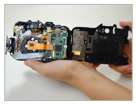
Open the back cover of the camera, see steps 1-6 in <u>Canon PowerShot</u> <u>G12 Rear Function Setting Dial</u> <u>Replacement</u>
