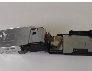
Flip the metal frame over to the left side of the camera and onto the surface on which you are working.
