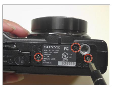
Remove all three screws from the bottom of the camera.
