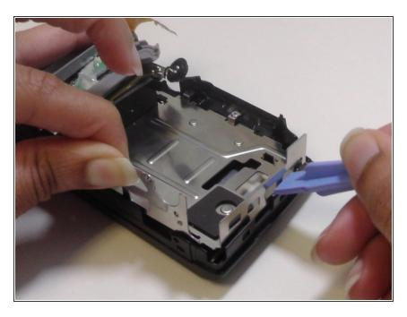
Use the plastic opening tool to assist you in separating the metal frame from the back cover of the camera.
