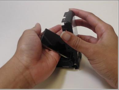
Now remove the LCD screen by bringing the back cover over to the left so that the LCD screen falls into your hand. To reassemble your device, follow these instructions in reverse order.
