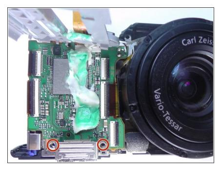
Remove the two screws from the bottom of the motherboard.
