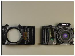
Pry the front cover of the camera off with the plastic opening tool.
