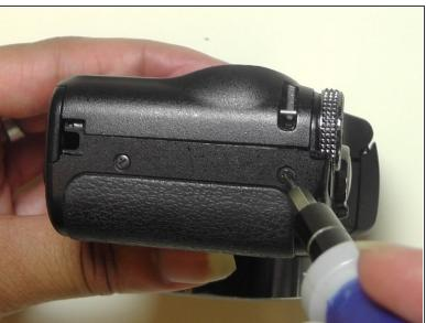
Remove the screws on the left and right sides of the camera.
