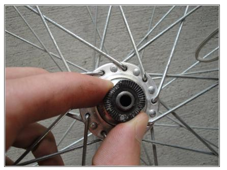
• Check the way that the axle spins in the wheel. The action should be smooth, with virtually no slop when wiggled. If it is to tight or too sloppy then you need to repeat the previous step.
