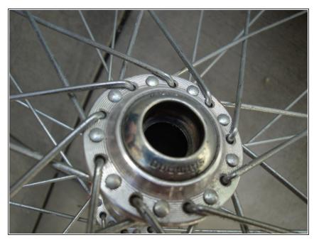
Clean bearings, the bearing races, and cones by wiping them off with a rag.
