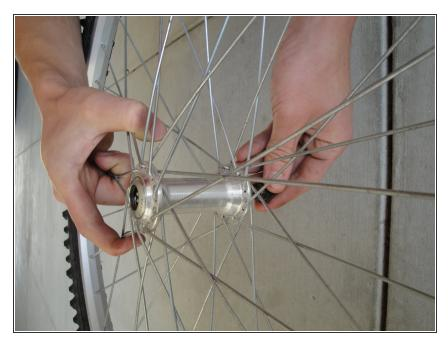
Insert the axle back into the wheel, with the still attached nut and cone on the bottom side of the wheel.
