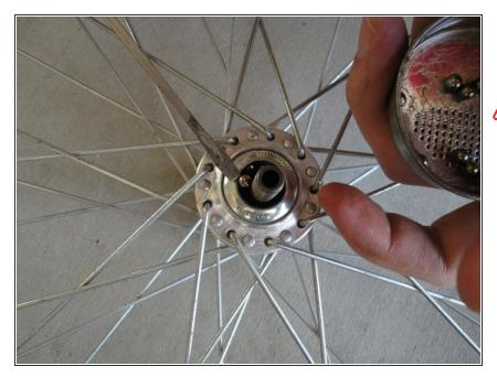
Insert 10 bearings into the topmost bearing races.
