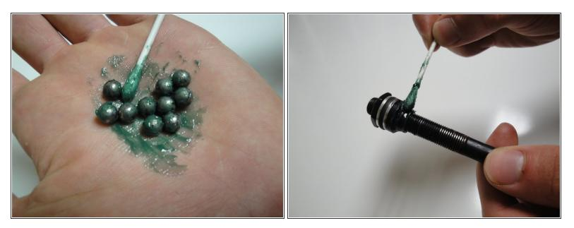
• Liberally apply grease to the bearings, races, and cones.
