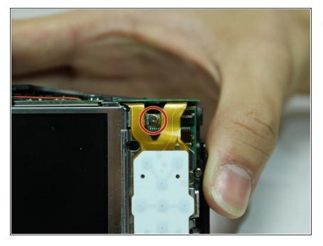
Remove the 3.9 mm screw with a Phillips #00 screwdriver.
