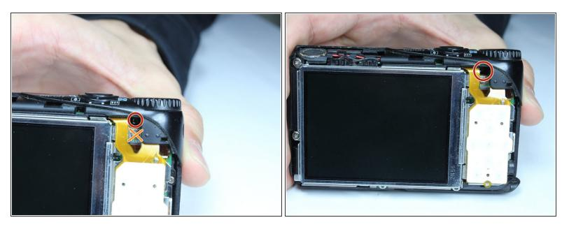
• Remove the internal 4.4mm screw with a Phillips 00 screwdriver.
