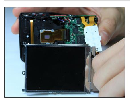
Holding the outer frame of the LCD screen, gently lift the LCD screen for replacement.
