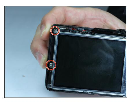
Remove the two 3.9 mm screws shown with a Phillips #00 screwdriver.
