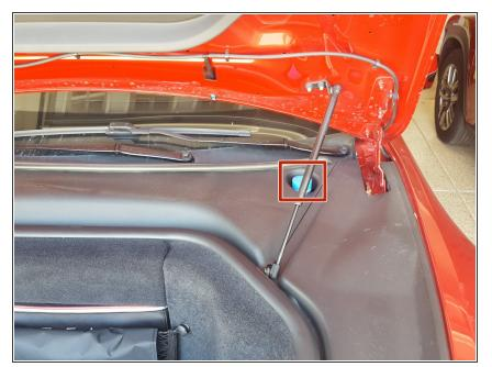
Remove the access cover just in front of the windscreen, it has a hole in it for WS washer fluid reservoir.
