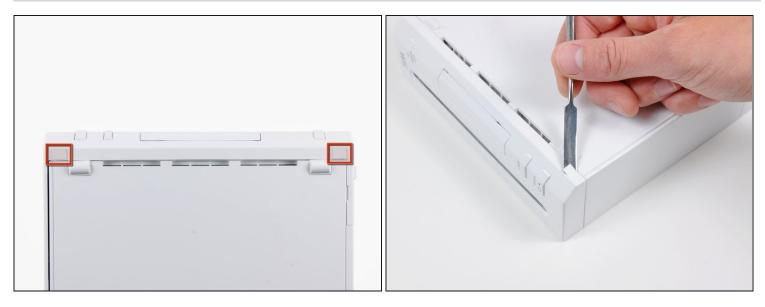
• Use a metal spudger to remove the white plastic screw covers stuck to the lower case near the front of the Wii.
