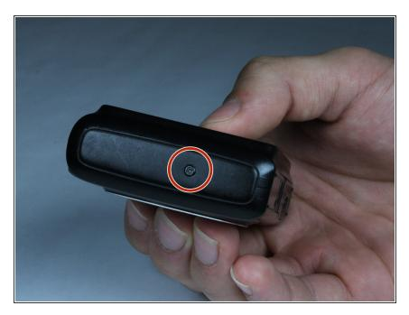
Remove the 5.0 mm screw on the left with a Phillips #00 screwdriver.
