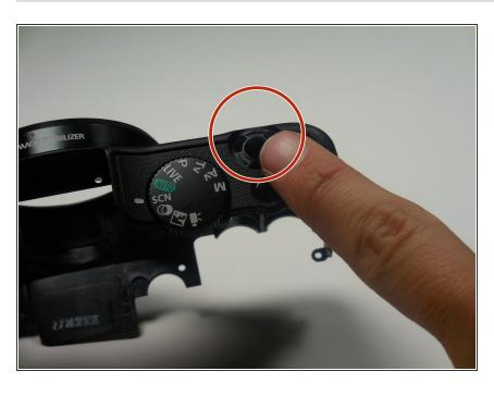
Locate and replace the shutter button on the front panel of the camera. Congratulations, you have successfully replaced your shutter button. To reassemble your device, follow these instructions in reverse order.
