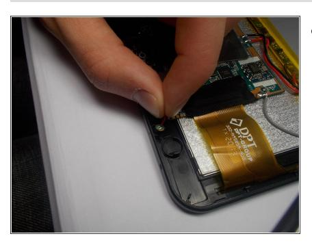
Grip the wires and slowly pull the microphone out of its mounting point. Some force may be needed.
