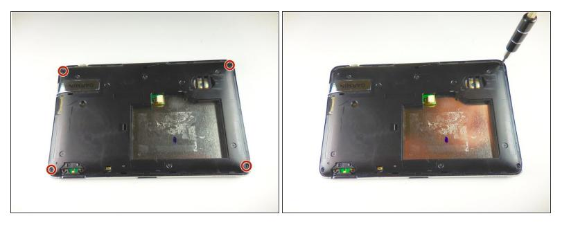
• Using the T5 bit, unscrew the four 5.7mm screws in the four corners of the device.
