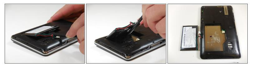
• Use the plastic spudger to lift the battery up and away from the device.
