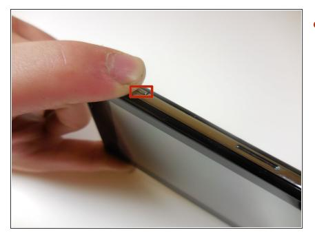
Turn the device off by pressing and holding the power button on the top left of the device.
