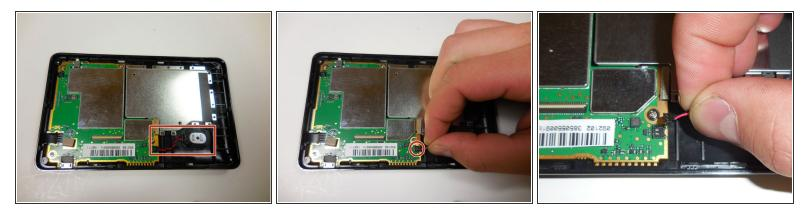
• Locate the red and black wire that connects the speaker to the circuit board. Use your fingers (or tweezers) to gently lift the plug off the circuit board.
