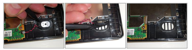
• With the plastic spudger, lift the speaker up and out of the frame.
