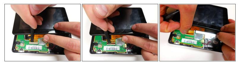
(i) For the larger orange connection, there is a white tab holding the connection to the circuit board.
