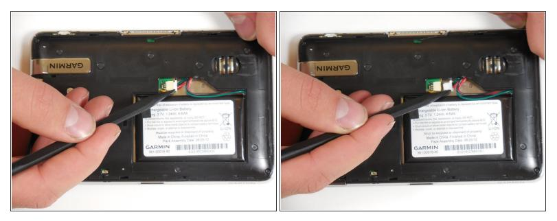
• Using the plastic spudger, carefully remove the white tab connected to the battery from the device by pulling the tab in the opposite direction from which it is connected.
