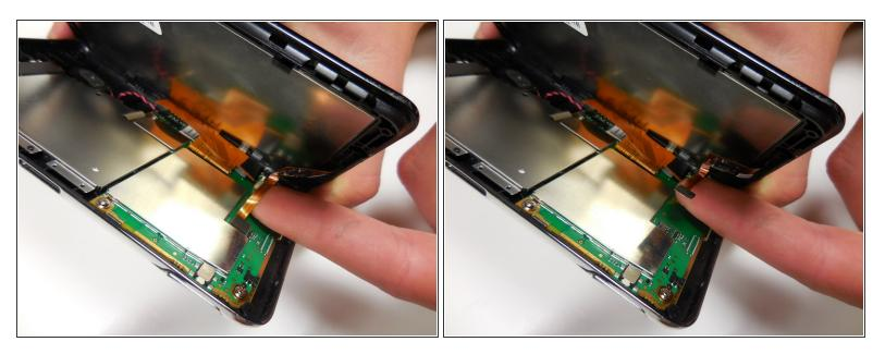
Pull up on the smaller orange tab with your finger from the circuit board. This connection will unplug with ease.
