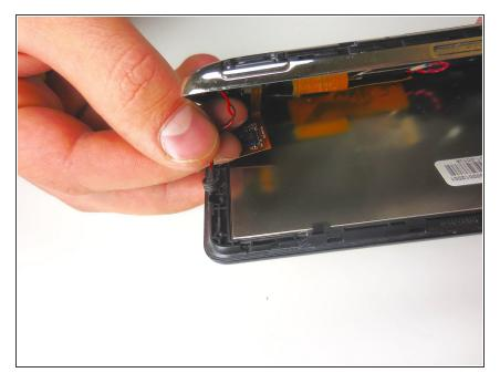
Using your fingers, remove the red and black wire from the back of the screen. This is the connection to the light sensor, not the speaker.
