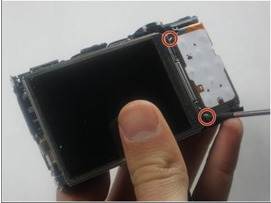
• Remove the 2 screws(1.95 mm) by the top right and bottom right of the screen.
