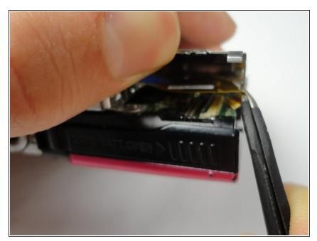
Gently remove the ribbon cable from the ZIF connector using the tweezers
