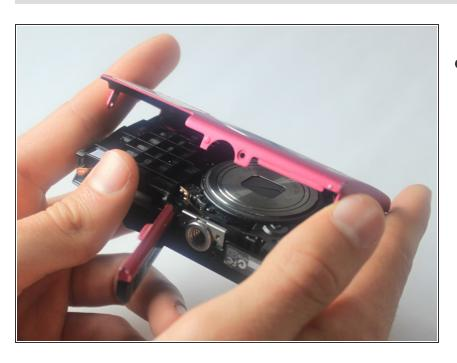
Gently lift the bottom of the front cover to roughly a 30 degree angle.
