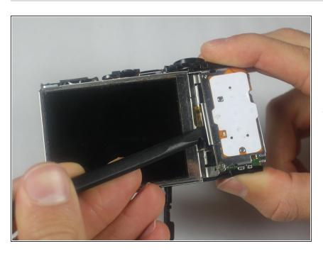
Wedge the flat end of the spudger between the camera and the function buttons plate to push the
