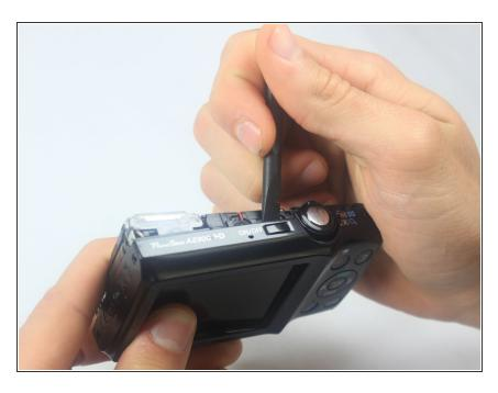
Pry the top off by sliding the spudger under the On/Off button.
