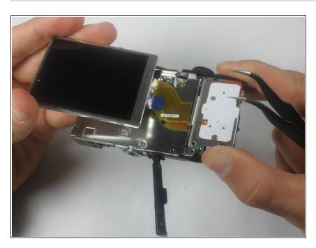
With the bottom of the function button plate still raised pull the screen out to the left until the ribbon cable is out from underneath the function button plate.
