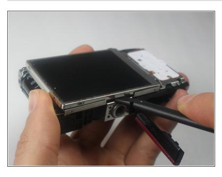
Raise the screen by wedging the spudger between the bottom of the screen and the mount hole.
