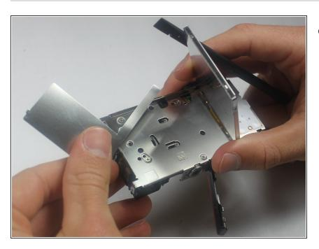
Remove the metal sheet that is under the screen.
