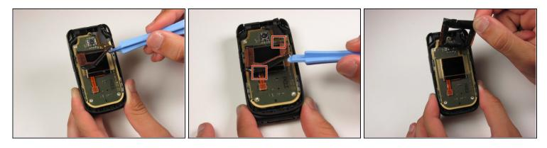
• Starting in the lower right corner, slowly begin to lift the tape that is holding down the front LCD and cables.
