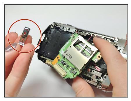
Remove the old record button from beneath the silver plate.
