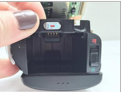
Place the new Record button into the open slot.
