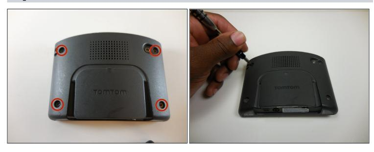
• Remove the 4 .4mm screws on the back of the device.
