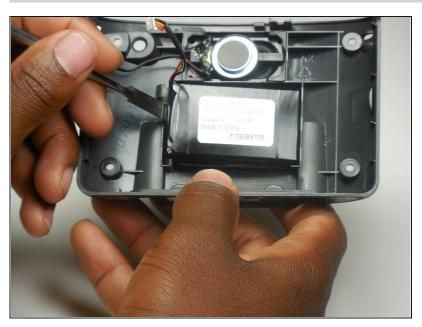
Using metal palate knife pry the battery from the back panel.
