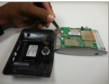
• Using the <u>tweezers</u> separate the wires connecting the battery and speaker to the mother board.
