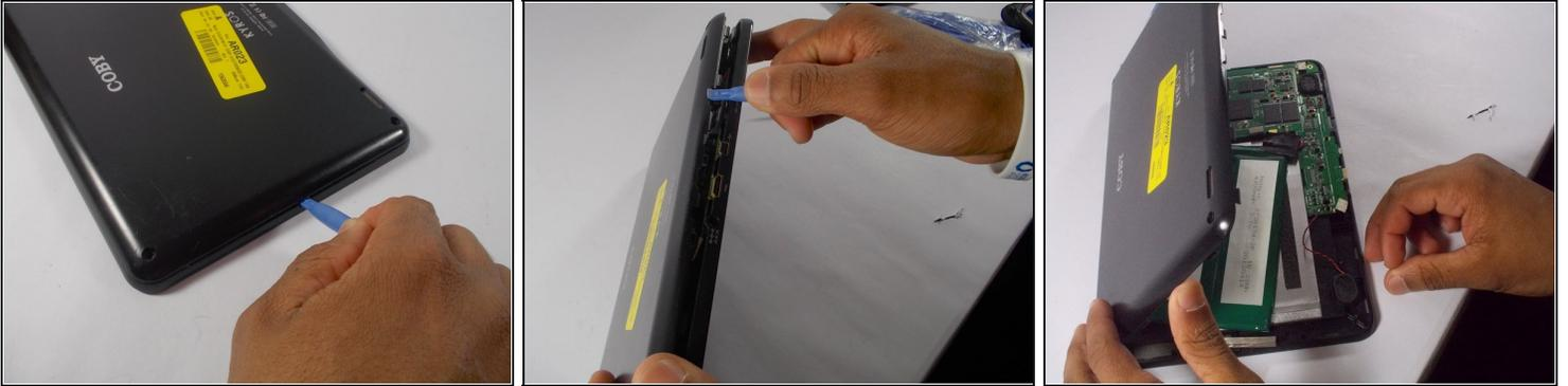
**⚠ Potential for device damage: Be careful not to break the inner plastic tabs while pulling the back cover off.**
