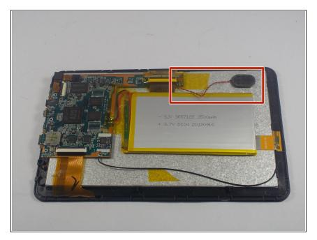
With the back cover removed from your tablet locate the speaker and the speaker wires shown in the red box.
