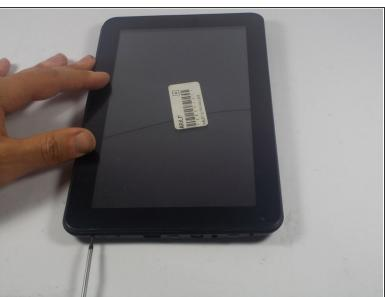
On the top of the tablet there are two 1cm screws that hold the back cover on. Locate these screws and remove them using a Phillips head #0 screw driver.
