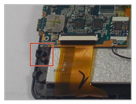
• You now have to remove the microphone from its original location. The microphone is in the small circular slot highlighted in the photo. If the microphone does not easily slide out you may need tweezers to remove it.
