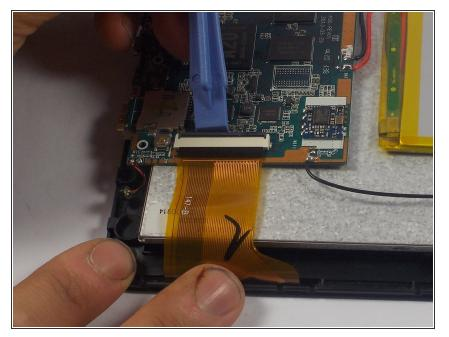
• There is a wire strip connecting the touch screen panel to the motherboard. This must be removed from the motherboard. To do this use a spudger to pry up the tab on the back of the connector. This will allow you to pull the wires out of the connection and will free the touch screen panel.
