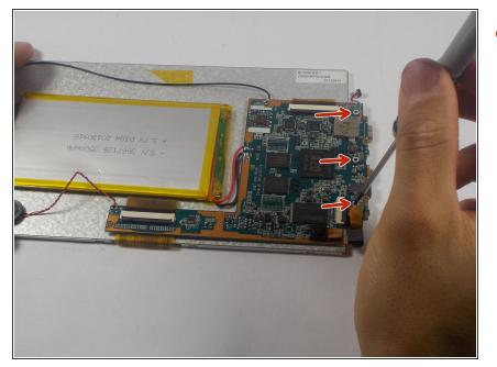
The first step is to remove the motherboard from the touch screen panel. To do this use a phillips head #0 screwdriver to remove the three 1cm screws that hold the motherboard to the panel. The screws are located at the top of the motherboard.
