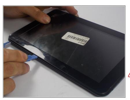
• You now have to pry the back cover from the touch screen panel. To do this insert a plastic spudger into the seem. Then work your way around the panel until it is free.
