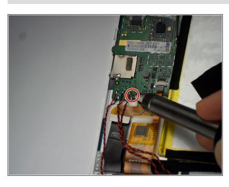
You will need a soldering/desoldering kit to <u>desolder</u> the 2 leads where the microphone connects to the circuit board. To reassemble your device, follow these instructions in reverse order.
