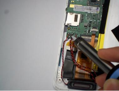
You will need a soldering/desoldering kit to <u>desolder</u> the 4 leads where the speakers connect to the circuit board. To reassemble your device, follow these instructions in reverse order.
