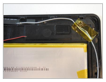
Remove tape from attached wire.
