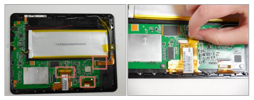
• Peel tape off of ribbon connectors. Starting at the power button, work clockwise around the tablet.
