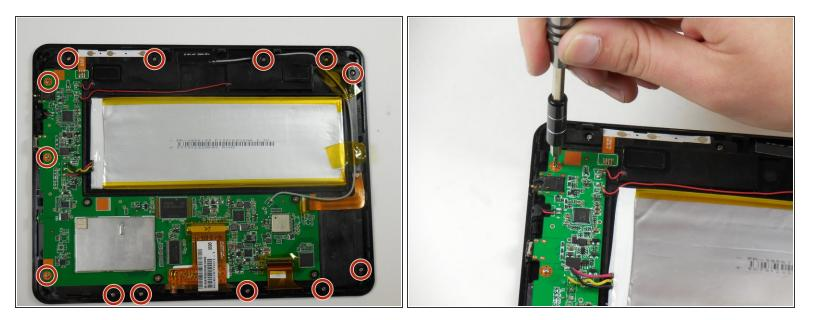
• Unscrew the thirteen 4.75mm screws around the perimeter of the tablet using a PH 00 screwdriver.
