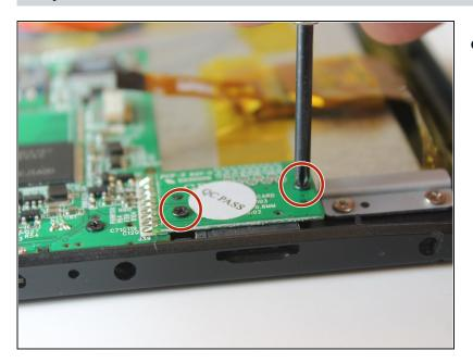
Remove the two screws that secure the micro-SD card reader to the tablet frame
