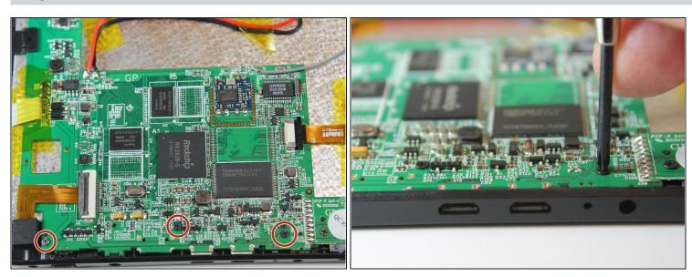
• Remove the three screws that secure the motherboard to the tablet frame
