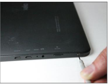
Remove the two 3 mm retaining screws from the side of the tablet with a Phillips #0 screwdriver.
