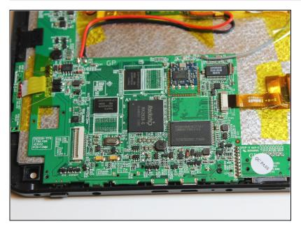
Place the motherboard back into its proper position but do not reinstall the securing screws yet.
