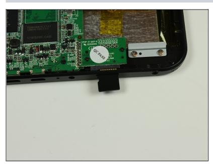
Remove the micro-SD card from the card slot if a card is in the slot
