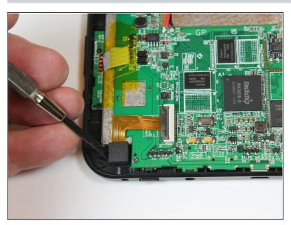
Remove the camera from its socket. Do not remove the camera ribbon cable.
