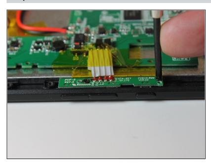
With the No. 0 Phillips head screwdriver, remove the two screw that hold the function and volume control switch assembly to the tablet.
