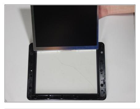
Pry up the LCD display and lift it away from the plastic screen.
